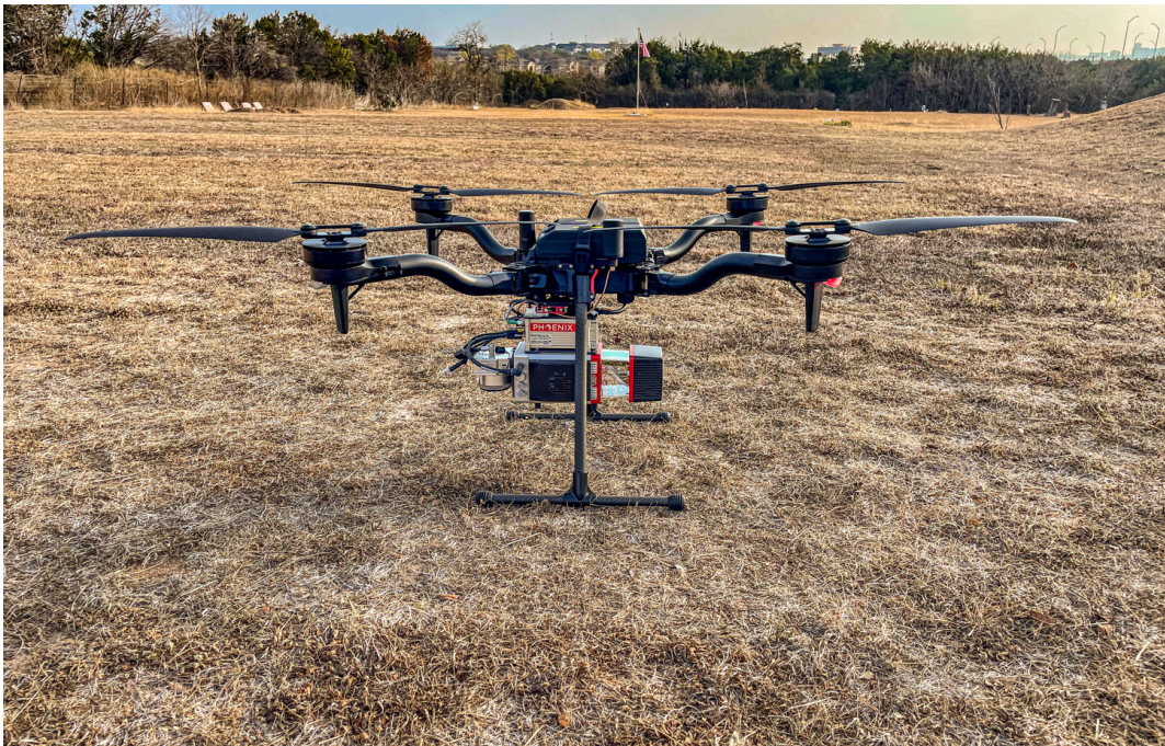
Fully Blue UAS-approved setup with the Freefly Astro Max and the miniRANGER-3 Lite. The miniRanger-3 was the first, and remains the longest-continuously approved, LiDAR payload on the Blue UAS list.
