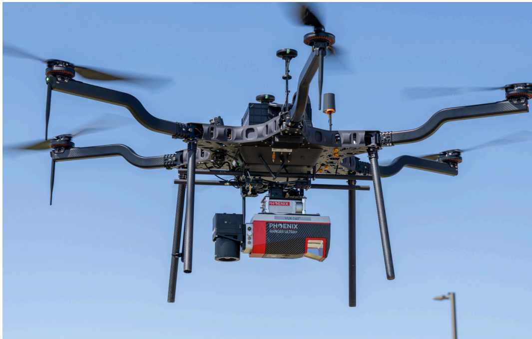
Ranger U-160 is a fully NDAA-compliant LiDAR system featuring a unique NFB field of view designed to deliver a high level of detail on vertical structures.
