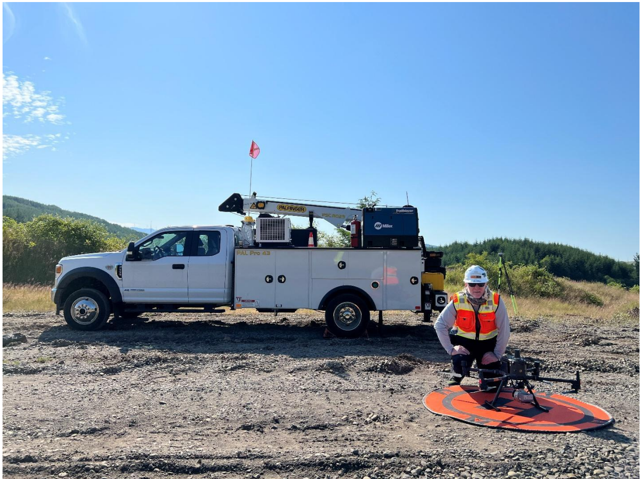
Pre-flighting the DJI M300 RTK and Phoenix LiDAR RECON-Xt at the Centralia Proving Ground
