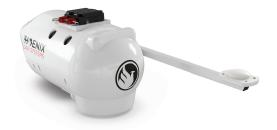
The **NEW ULTRAPOD** from Phoenix LiDAR Systems is a complete, turn-key, aerial solution designed to adapt to a wide range of mapping and survey missions. This lightweight and robust composite housing is FAA and EASA approved for Cessna 172, 182, and 206 aircraft, giving operators a userfriendly, flexible mounting solution for LiDAR payloads and cameras.
