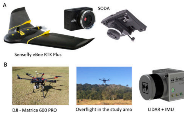
Fig. 2. (A) Sensefly fixed-wing eBee RTK Plus + SODA camera; (B) DJI Matrice 600 Pro + LIDAR system, both used in the experimental site, in July/August 2017.
