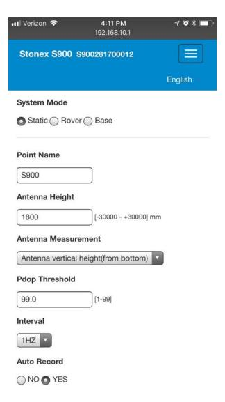
Note: By selecting "Auto Record: Yes", the next time you power on the S900, it will begin recording static data (using the established configuration above) once it has a solution status.
