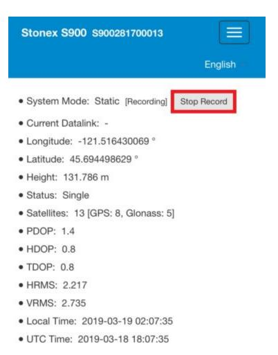
Note: Once you power off the S900 receiver head, the Static working mode configuration is stored. This configuration will be applied to future static sessions (when receiver head is powered back on) until the configuration is changed.
